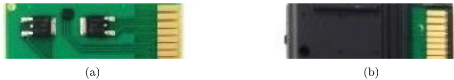
Figure 5.5.8: ECU configurations. (a) Unmolded configuration. (b) Molded configuration.
