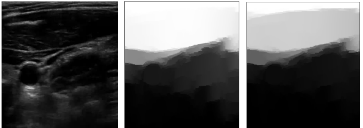
Figure 4.14: Different values of \alpha can affect the confidence map (a) US image, (b) \alpha = 2 , (c) \alpha = 6
