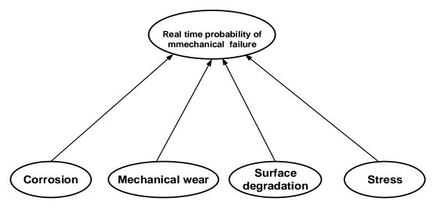
Figure 6. 2. Probabilistic networks structure of causes of mechanical failure generated from historical data.
