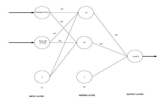
Figure 7. 2 – Schematic diagram of ANN architecture of flow system of a tank.
