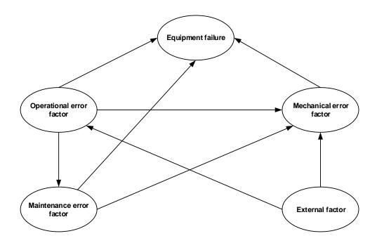
Figure 4.6. Interdependency of accident contributory factors in Equipment failure prevention barrier.
