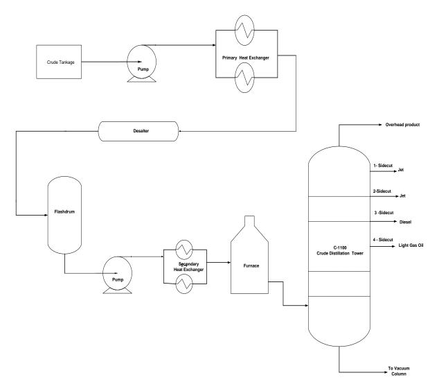
Figure 8.2. The process flow diagram of Richmond refinery crude unit and it associated up stream equipment( Adedigba et al. 2016; CSB 2015).
