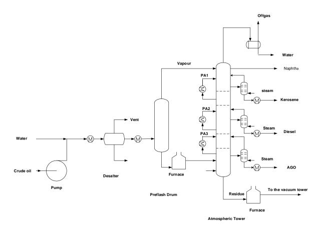
Figure 6. 5. Process flow diagram of the crude distillation unit. (Al-Mayyahi et al. 2014).
