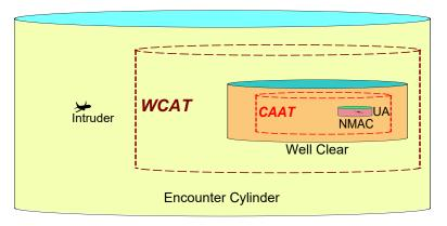
Figure 4.2: Layered encounter model of the airspace nearby the UA.
