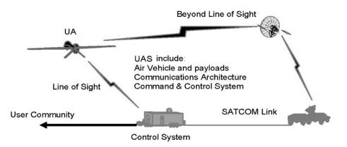
Figure 1.1: A typical system diagram for UAS [3].
