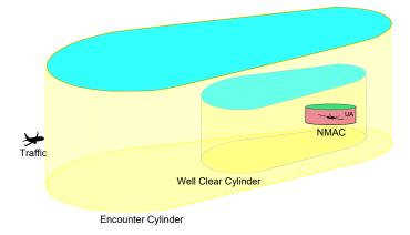
Figure 2.12: A dynamic-size encounter cylinder in the three-dimensional space.
