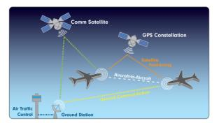
Figure 2.4: ADS-B surveillance configuration diagram [7].
