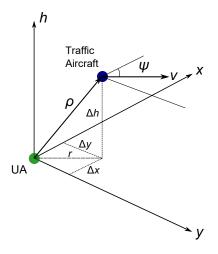
Figure 2.9: Aircraft positions in the three-dimensional space [9].
