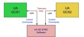
Figure 7.5: UA 4D synchronization system schematic diagram
