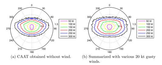
Figure 4.14: Summarized range-based CAAT diagrams (bearing in deg, range in nmi, UA at 75 kt vs. traffic at various airspeeds).
