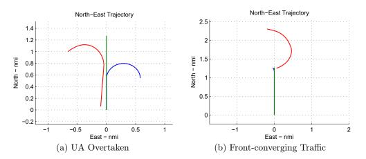
Figure 6.18: Sample diagrams for unresolved NMAC encounters in risk ratio analysis due to system delays.
