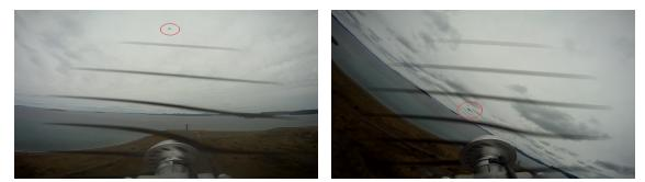
(a) No maneuver required for traffic UA on the top (b) Left turn maneuver triggered for a co-altitude traffic UA in the front
