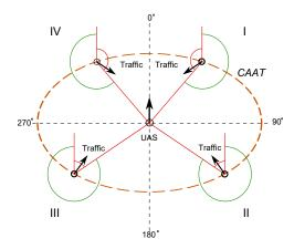
Figure 6.8: Horizontal maneuvering strategies in the three-dimensional evasive maneuvering algorithm.
