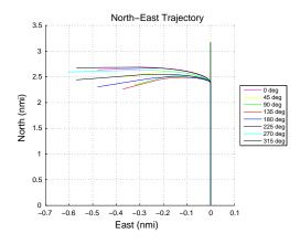
Figure 4.6: Sample turning trajectories for 75 kt UA under 20 kt winds in various wind directions from 0° to 360° every 45° by 20-second 2g left level turns (6°/sec).
