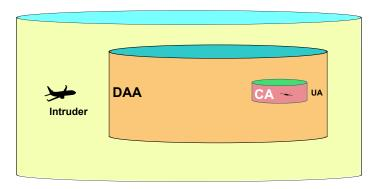
Figure 1.3: Diagram for DAA and CA regions in a mid-air encounter.
