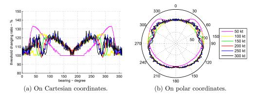
Figure 4.15: Threshold changing ratio diagrams for the impact of CAAT boundaries on wind uncertainties (UA at 75 kt vs. traffic at various airspeeds).
