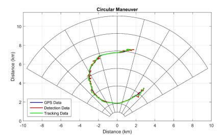
Figure 7.20: Results for the circular maneuver [14]. Distances are relative to the radar, bearings are relative to the  $80^{\circ}$  radar pointing angle, the range rings interval is 1 nmi and the scan spoke interval is  $15^{\circ}$ .
