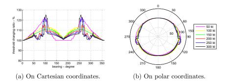
Figure 4.12: Threshold changing ratio diagrams for the impact of WCAT boundaries on wind uncertainties (UA at 75 kt vs. traffic at various airspeeds).
