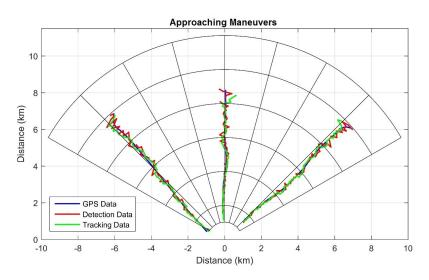
Figure 7.18: Results for the approaching maneuvers [14]. Distances are relative to the radar, bearings are relative to the  $80^{\circ}$  radar pointing angle, the range rings interval is 1 nmi and the scan spoke interval is  $15^{\circ}$ .
