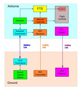
Figure 7.22: System configuration for BVLOS UAS.
