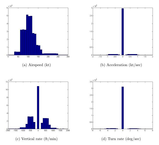
Figure 2.14: Feature histograms of five million sample encounters simulated on the fast-time simulation platform.
