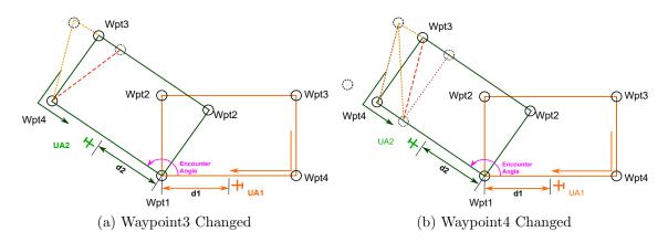
Figure 7.6: UA 4D synchronization system design diagram.
