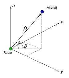
Figure 3.2: Radar polar and Cartesian coordinates diagram [11].
