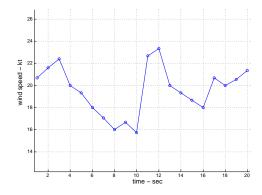
Figure 4.9: An example of 20-second gusty wind pattern with wind velocity jumps [12].
