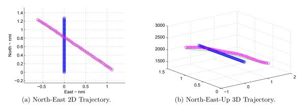
Figure 3.7: A pair of sample encounter trajectories estimated by EKF through ground portable radar measurement. (Legend: blue for simulated UA trajectory, green for simulated traffic true trajectory, and magenta for estimated traffic trajectory.)
