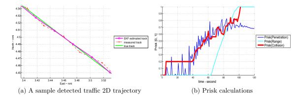
Figure 5.8: Diagrams of  $P_{risk}$  calculations based on sensor measurements.
