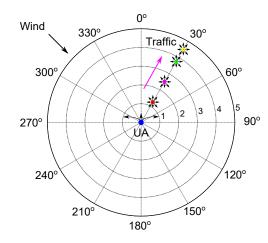
Figure 4.8: A web structure for Monte Carlo simulations to determine WCAT and CAAT boundaries (bearing in deg and range in nmi).
