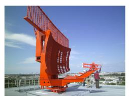
Figure 2.1: Antennas of a typical ground surveillance radar system for ATC [4].
