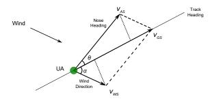
Figure 4.7: Aircraft trajectory generation in the wind.
