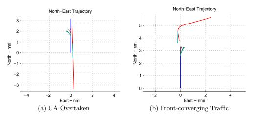
Figure 6.16: Sample diagrams for unresolved LoWC encounters in risk ratio analysis due to system delays.
