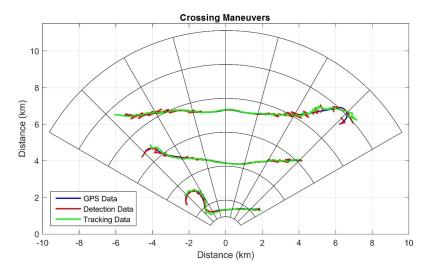
Figure 7.19: Results for the crossing maneuvers [14]. Distances are relative to the radar, bearings are relative to the  $80^{\circ}$  radar pointing angle, the range rings interval is 1 nmi and the scan spoke interval is  $15^{\circ}$ .
