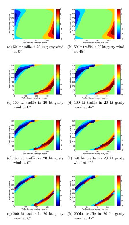
Figure 6.4: Sample policy network diagrams for UA maneuvering options in various velocities and wind conditions (UA: velocity at 75 kt and heading to the north; Legend: negative indexes for left turns in cool colors and positive indexes for right turns in warm colors).
