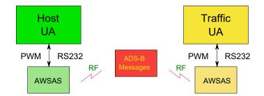
Figure 7.9: Cooperative ADS-B based ACAS schematic diagram.
