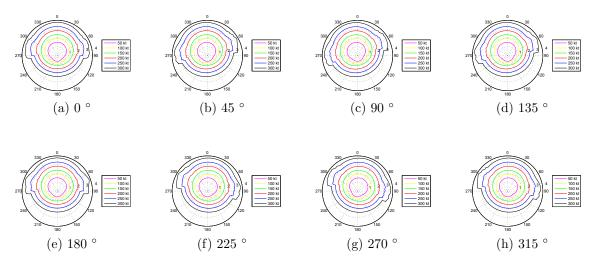
Figure 4.10: Range-based WCAT diagrams with 20 kt gusty winds in eight directions (bearing in deg, range in nmi, UA at 75 kt vs. traffic at various airspeeds).
