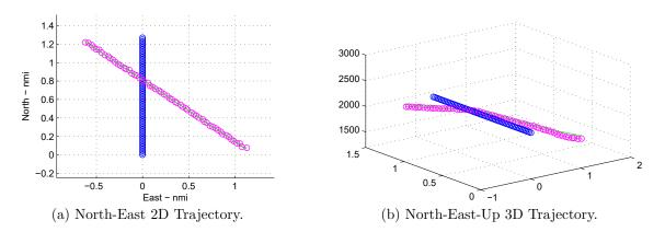
Figure 3.6: A pair of sample encounter trajectories estimated by EKF through ADS-B measurement. (Legend: blue for simulated UA trajectory, green for simulated traffic true trajectory, and magenta for estimated traffic trajectory.)
