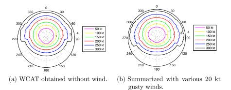
Figure 4.11: Summarized range-based WCAT diagrams (bearing in deg, range in nmi, UA at 75 kt vs. traffic at various airspeeds).
