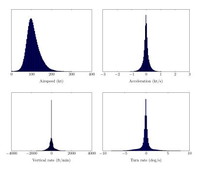
Figure 2.11: Feature histograms of recorded radar data based on 193 million samples [10].
