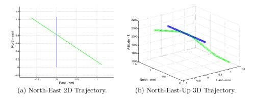
Figure 2.13: A pair of sample encounter trajectories generated by the uncorrelated encounter model (legend: blue for UA and green for traffic).
