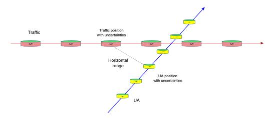
Figure 3.4: Aircraft measured positions with uncertainties during mid-air encounters.
