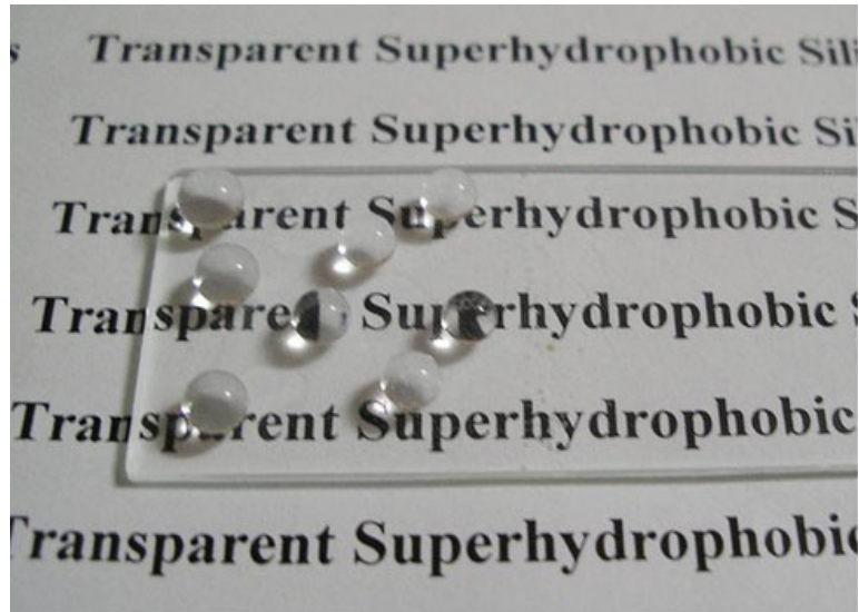
Figure 2.19 The Optically Transparent Superhydrophobic Glass Surface from Sol-gel Method
