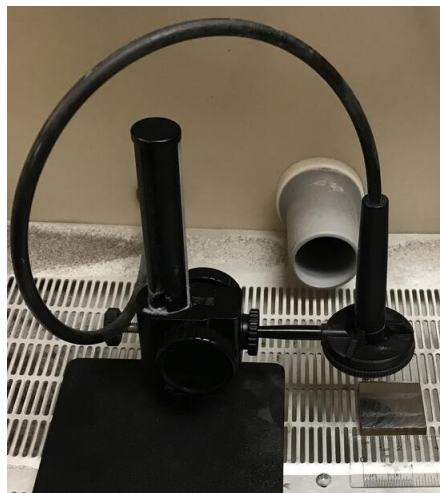
Figure 4.2 The Spray Gun Holder
