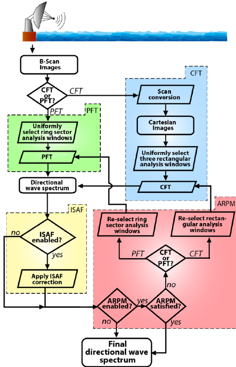
Figure 6.1: Flow chart of the directional wave spectrum estimation using the PFT, ARPM and ISAF. The blue, green, yellow, and red boxes highlight the standard CFT, the PFT, the ISAF and the ARPM methods, respectively.
