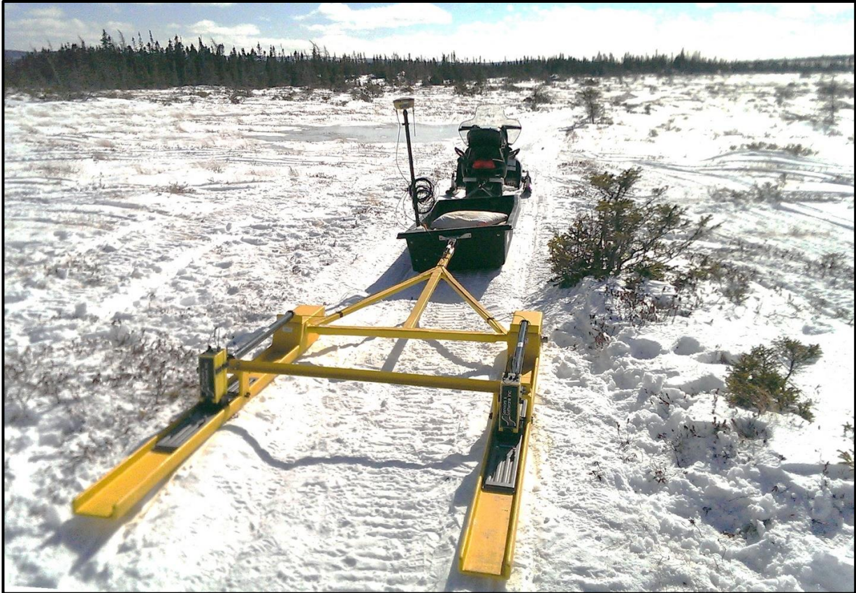
Figure 3.4: Configuration of GPR survey components including snowmobile, sled for the operator and RTK mount, and skis for housing the transmitter and receiver.
