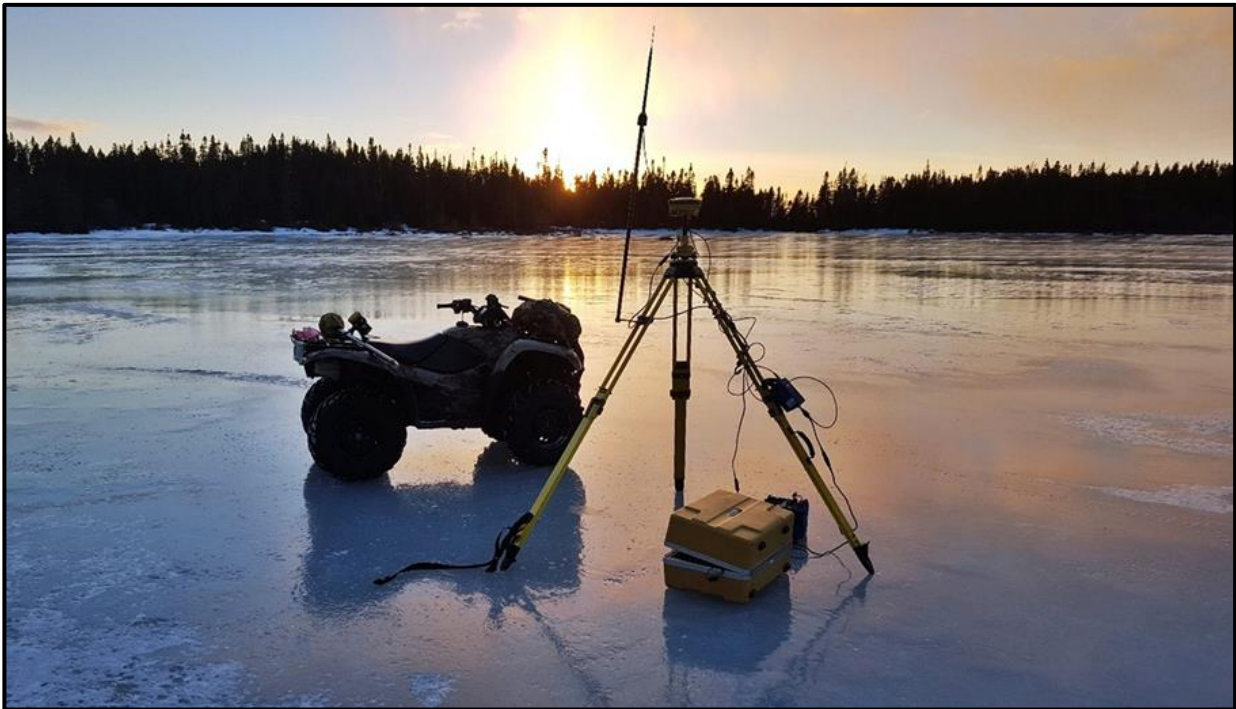
Figure 3.7: Setup of the RTK base receiver. System consists of receiver (on top of tripod), external battery (behind yellow case), and the radio which consists of the amplifier (right leg) and antenna (left leg). See Figure 3.4 for roving receiver).
