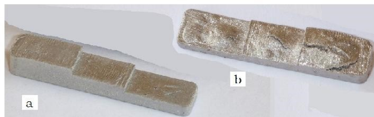
Figure 5: Sintered Part a) without and b) with defects.
