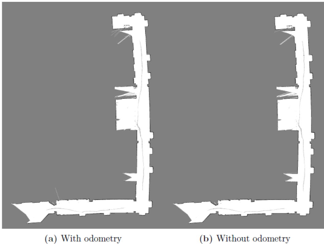
Figure 2.9: The resulting maps with and without odometry, both with identical LiDAR data (Berg, 2013).
