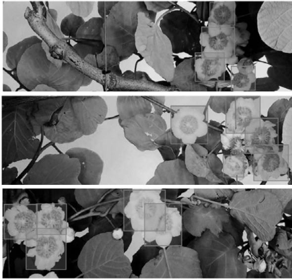
Figure 5 - Machine vision detection of kiwifruit flowers in real-world orchard environment
