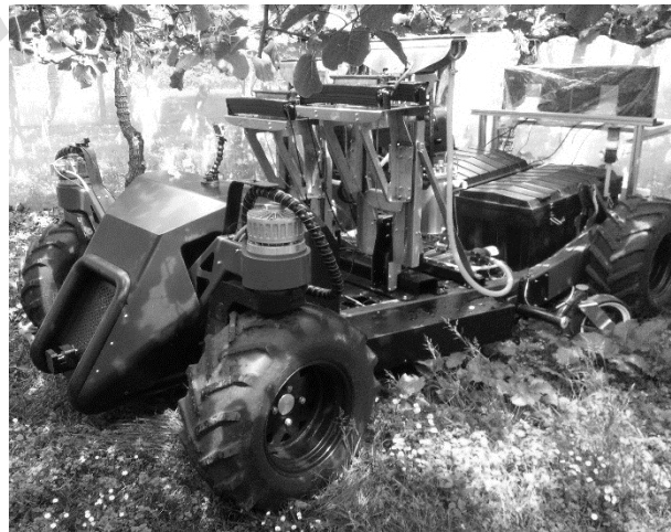
Figure 4 - Pollination system mounted on AMMP during experimental orchard trials
