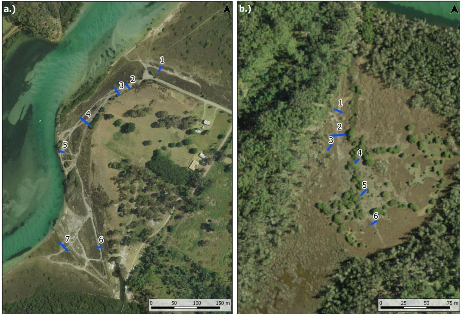
Figure 17: Location of transects intersecting vehicle tracks, at a.) Bermagui and b.) Tomakin, used to spatially analyse variation in elevation and micro-topography in response to disturbance
