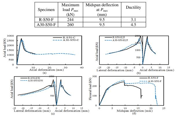
Table 2 Summarise test results of specimens testing under four-point bending
