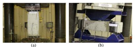
Figure 1. Test setup: (a) Axial compression and (b) Four-point bending
