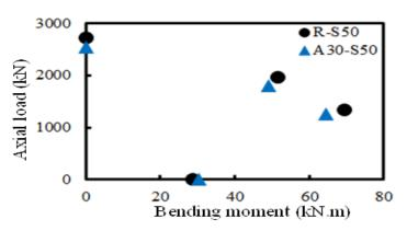
Figure 3 Experimental axial load-bending moment interaction diagram of specimens
