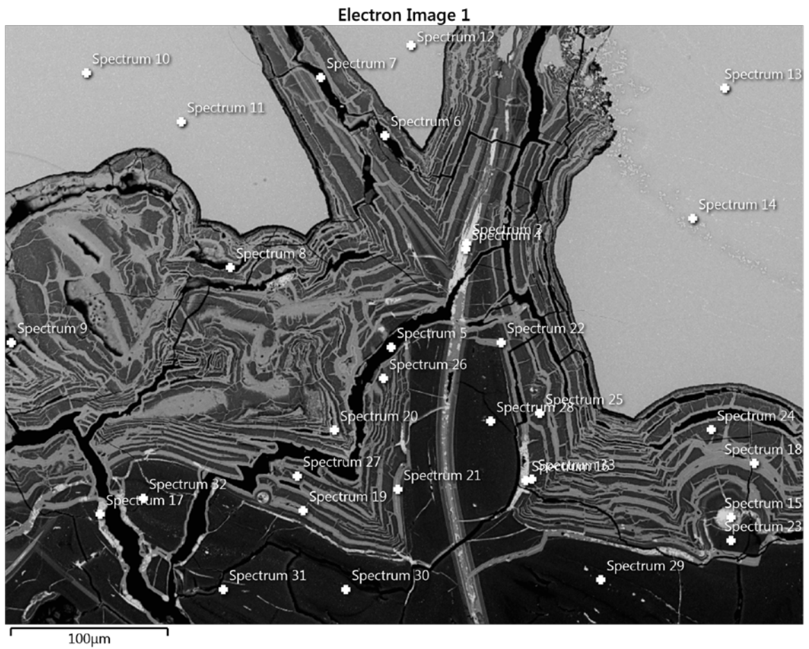
Figure 49: Image of sample MD obtained using a scanning electron microscope (SEM) showing locations of different spectra analysed using EDS
