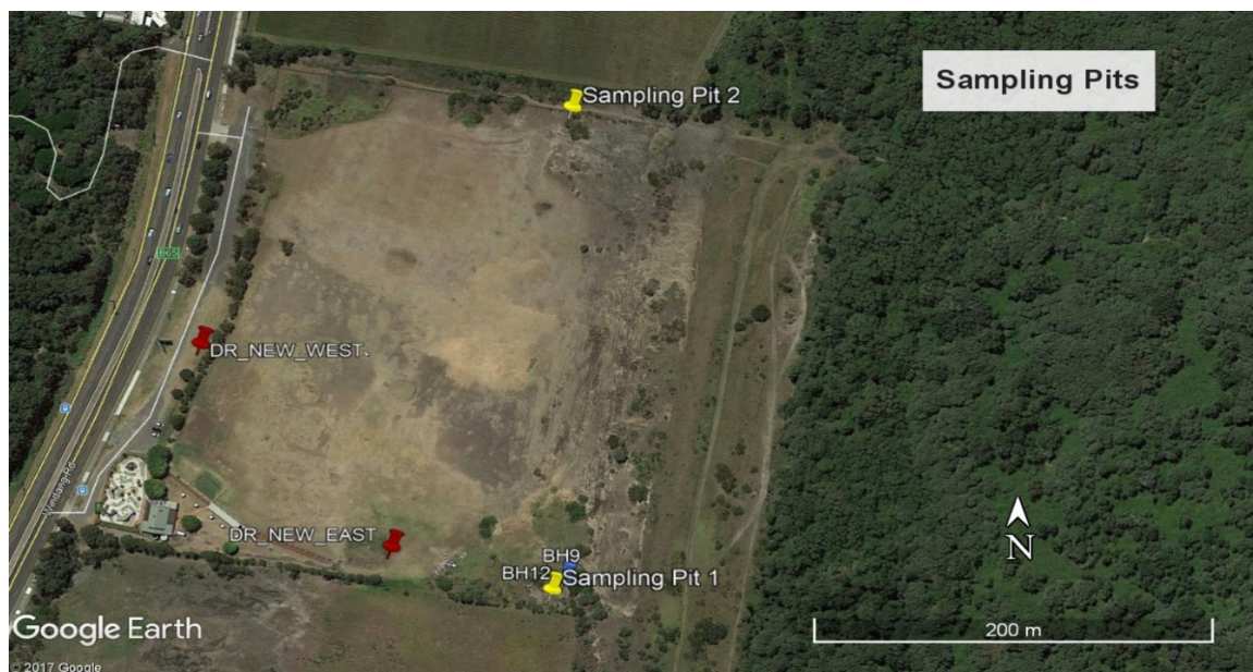
Figure 14: Location of sampling pit (b) (Figure 15) and sampling pit (c) (Figure 16) which were dug in order to collect slag samples from layers with variable levels of weathering. Descriptions of each pit are displayed in Table 4
