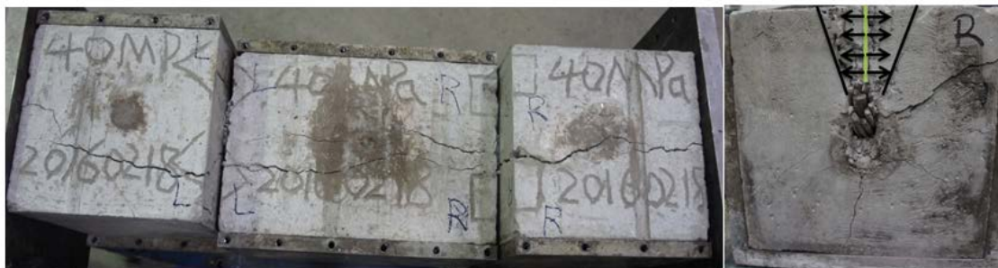
Figure 5: Double shear post-test concrete blocks crack
