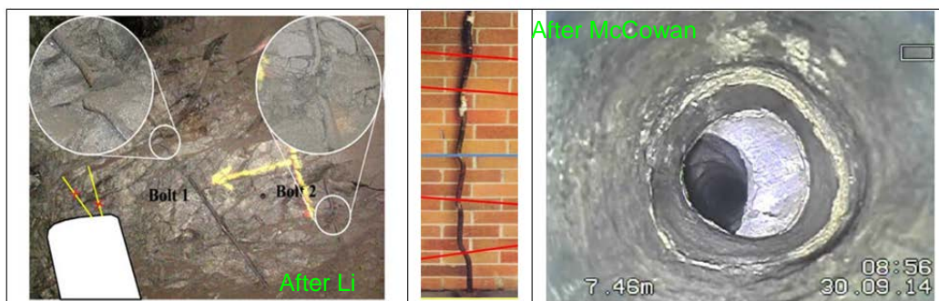
Figure 1: Sheared tendons recovered from field and a hole view of sheared rock (McCowan, 2015 and Li, 2017)
