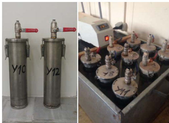
Figure 3: A view of desorption canisters in water at 28^\circ\text{C} reservoir temperature.
