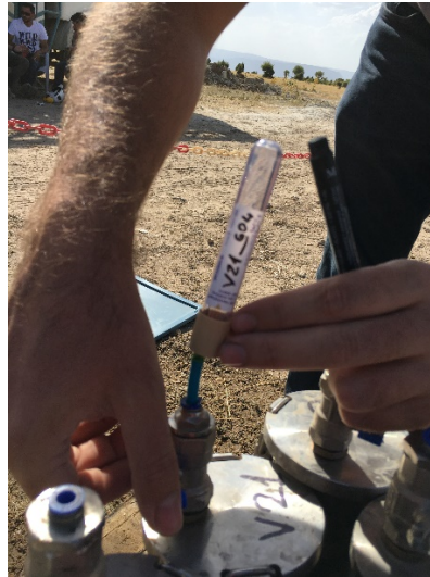
Figure 4: Gas sampling at the field using vacutainers.
