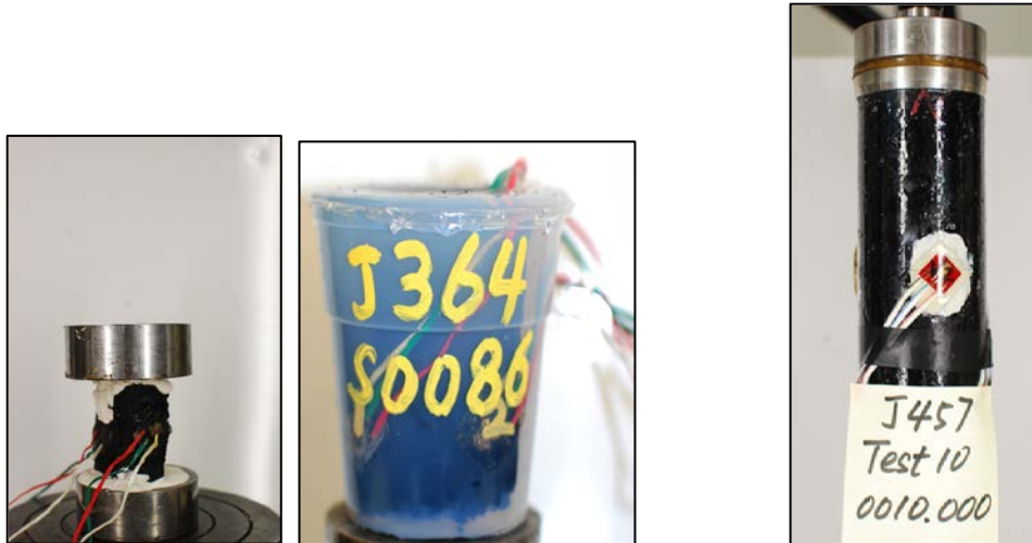
Figure 1: Coal sample for uniaxial test (left), and coal fragment for hydrostatic test (middle) and triaxial test (right).
