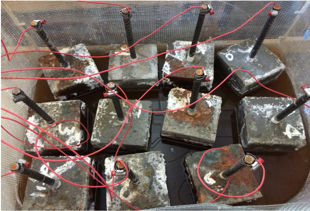
Fig. 4. Specimens during accelerated corrosion test.
