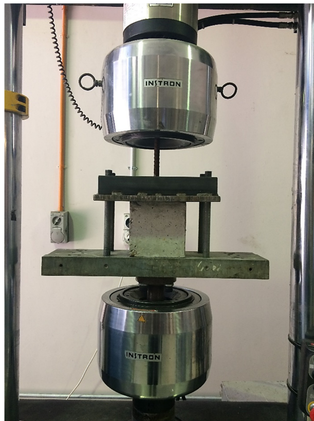
Fig. 5. Pull-out test: (a) Schematic diagram and (b) Actual setup.
