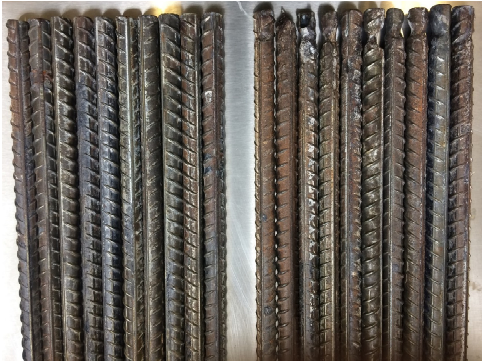
Non-corroded reinforcing steel bars Corroded reinforcing steel bars
