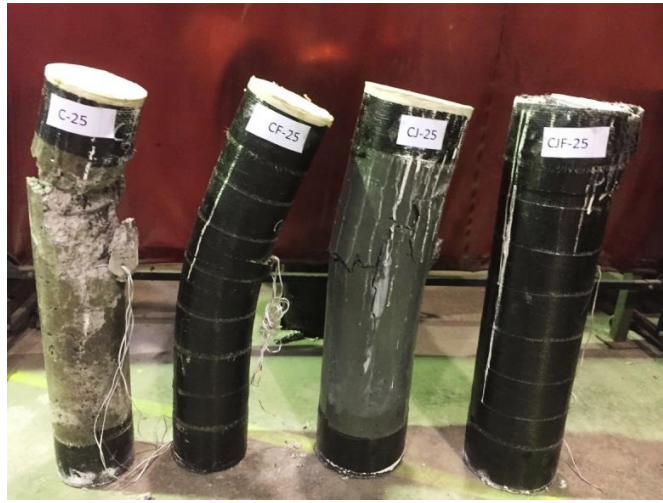
857 Fig. 11. Failure modes of the specimens tested under eccentric axial load (eccentricity = 25 mm)
