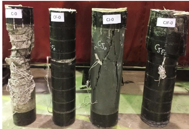
Fig. 7. Failure modes of the specimens tested under concentric axial load
