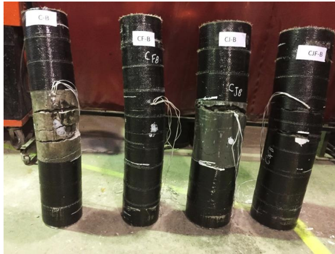
Fig. 13. Failure modes of the specimens tested under four-point bending
