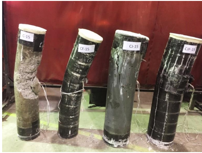
840 Fig. 9. Failure modes of the specimens tested under eccentric axial load (eccentricity = 15 mm)
