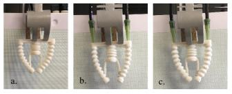
Fig. 6. Experimental results: a. The soft gripper without stiffenning wall was actuated by vacuum only in the middle bellow, b. The soft gripper with stiffenning wall was actuated by vacuum only in the middle bellow and c. The soft gripper with stiffenning wall was actuated by vacuum only in the middle bellow and pressure in the finger bellows.
