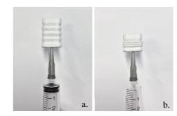
Fig. 3. A 3D printed airtight bellow sample a. in it is neutral state and b. in its under-vacuum state.
