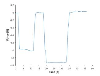
Fig. 7. Blocking force measurements and stiffening effect (Blocking force measurement test rig is presented on the photo (force values are in compression).
