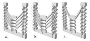
Fig. 1. Soft monolithic gripper designs: a. a halved model of the gripper without stiffening wall, b. a halved model of the gripper with stiffening wall and c. a halved model of the gripper without stiffening wall with one interconnecting-link.
