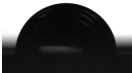
Figure S16. Shape of a water droplet on the flat SMP surface with a contact angle of about 84^\circ .
