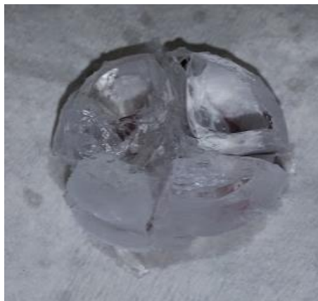
Figure 3.7: Microfibre ice ball after impact
