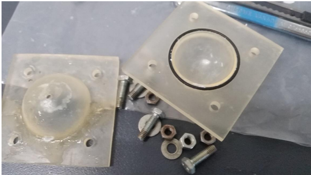
Figure A.2: 3D printed sphere mould (two halves)
