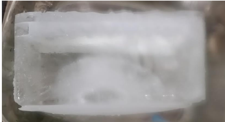
Figure A.3: Ice block containing the mould filled with water
