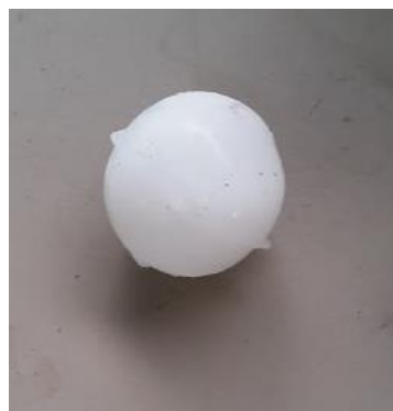
Figure 3.9: Intact artificial hailstone made with 12% PVA after the impact test
