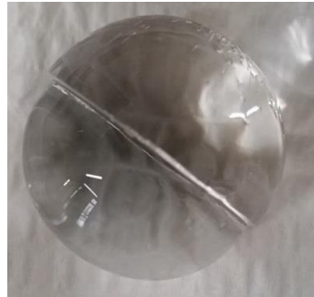
Figure 3.5: Pure ice ball free of air and cracking
