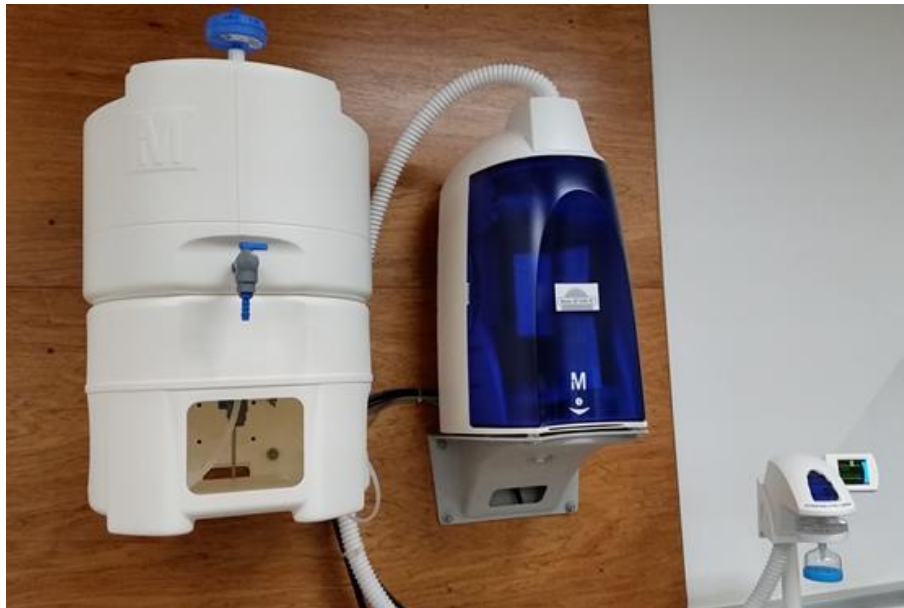
Figure 3.8: Water purification system used to produce demineralized water
