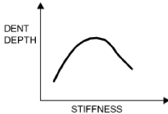
Figure 2.7: Relationship between stiffness and dent depth for static loading (Werner 1993)
