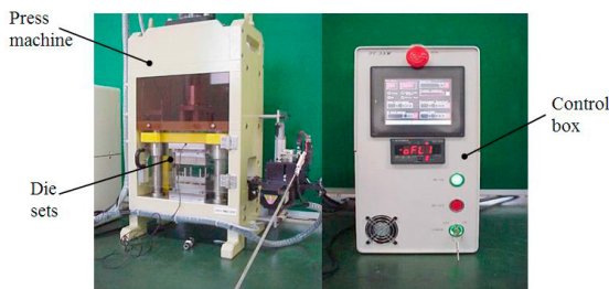
Fig. 4. Desk-top servo press machine DT-3AW.
