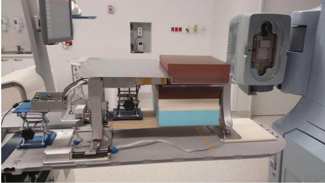
Figure 53: Setup for the moving target test with the detector placed on a movable tray.
