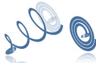
Fig. 1 Representation of a PPyEAP robotic bacterium (in its initial state in the right image and in its fully actuated state in the left image).
