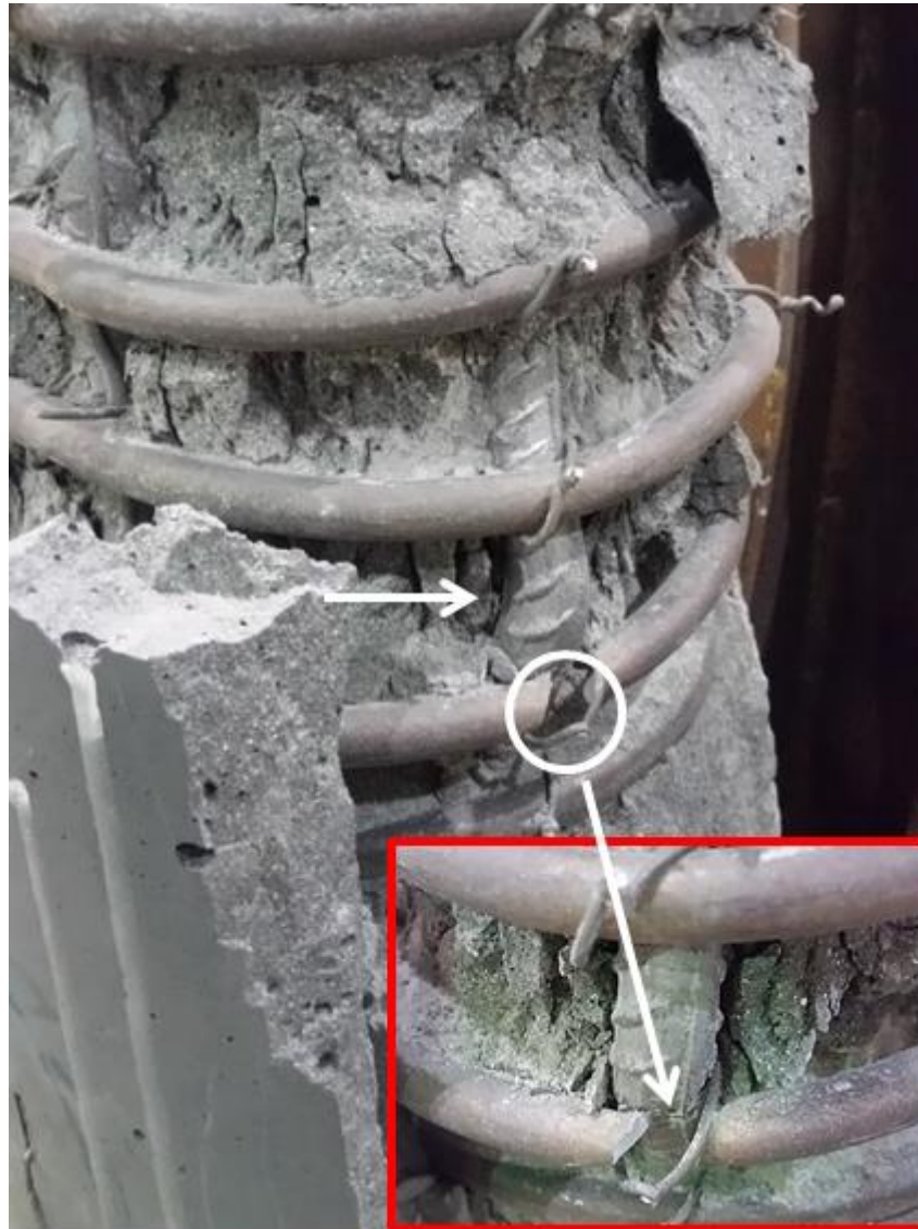
876 Fig. 6: Buckling of the longitudinal steel bar and rupture of the confining helix of Specimen
