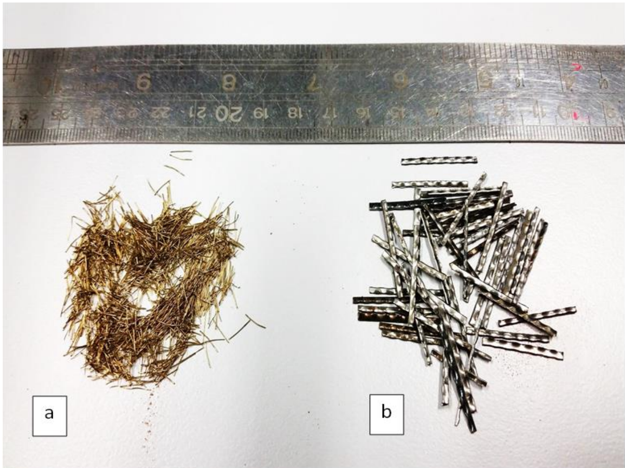
Fig. 1: The utilized steel fibres: (a) Micro steel fibre (MF); (b) Deformed steel fibre (DF).
