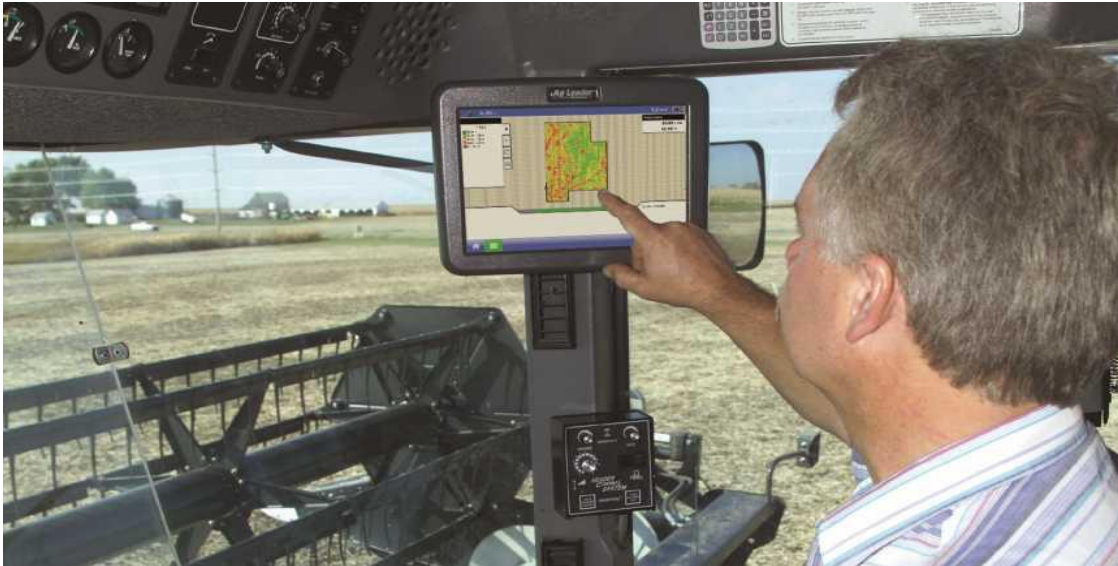
Figure 2: Pictured above is a yield monitor that a farmer is using to locate a specific field. (Heacox, 2015)
