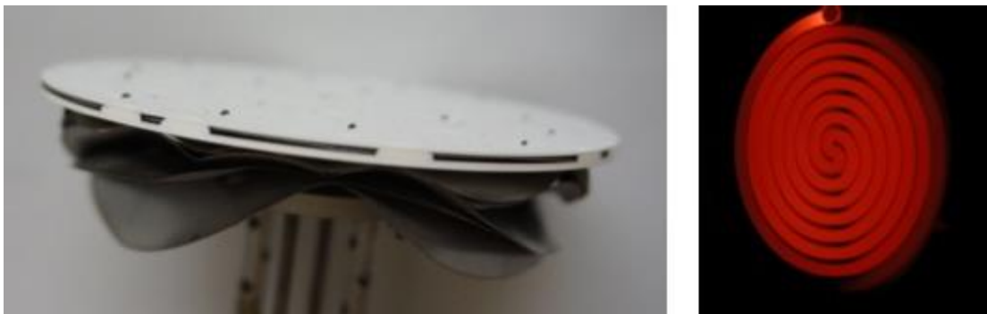
Figure 21. Tantalum heater (left) oxidizes while SiC (right) can operate in high heat and oxygen.
