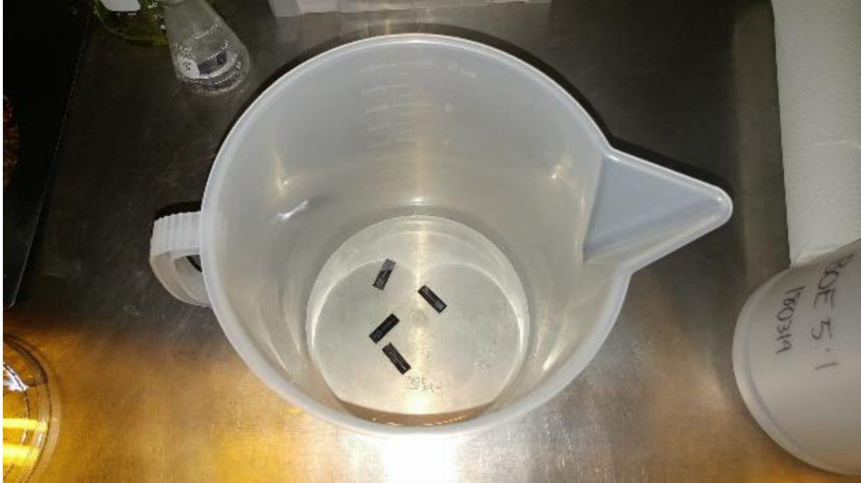
Figure 23: Buffered oxide (BOE) 5:1 was used to etch a 1000nm silicon oxide layer to expose the silicon wafer in a desired mask pattern.
