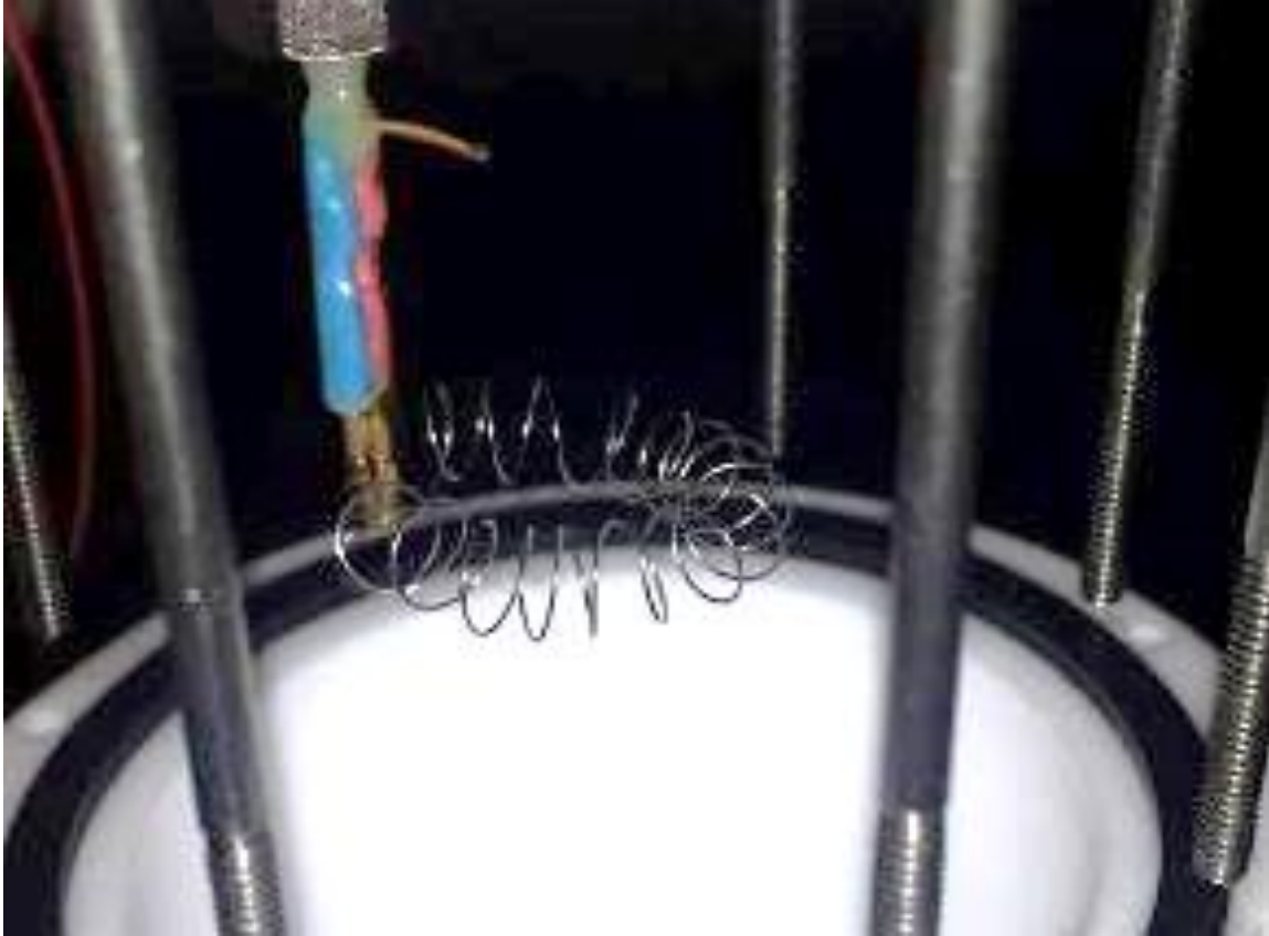
Figure 37: A coiled nichrome wire maintained constant aqueous antifreeze solution temperature during experimental trials.
