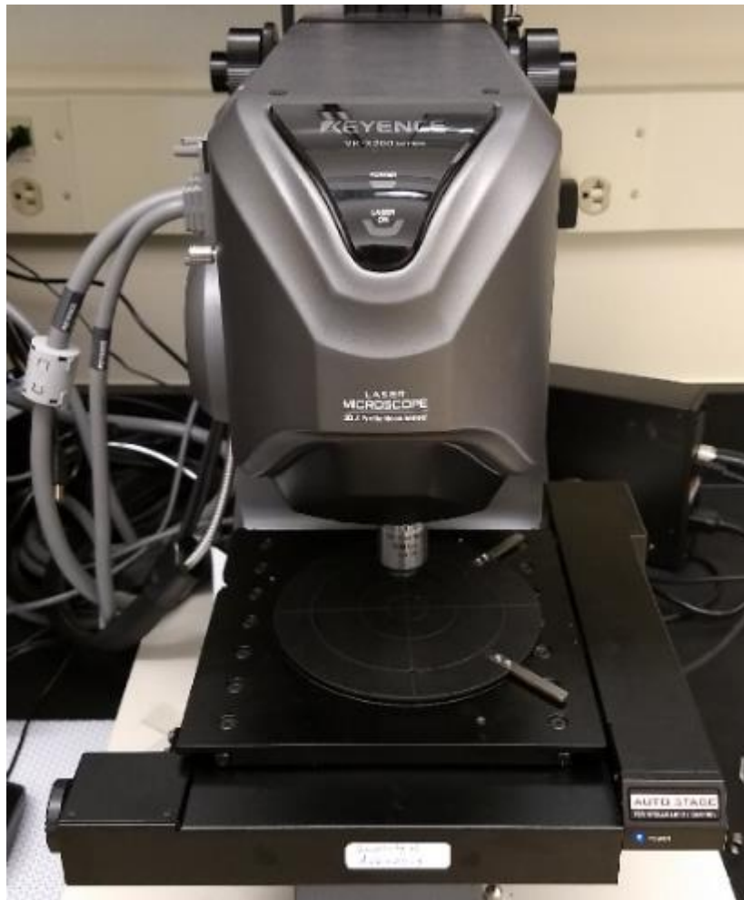
Figure 71: A Keyence X200 laser profilometer measured the channels in three dimensions. The laser scanned individual pixels and based on intensity readings determined a Z-height. Entire channels are scanned at once to visualize any defect that might inhibit flow in the nanochannel.
