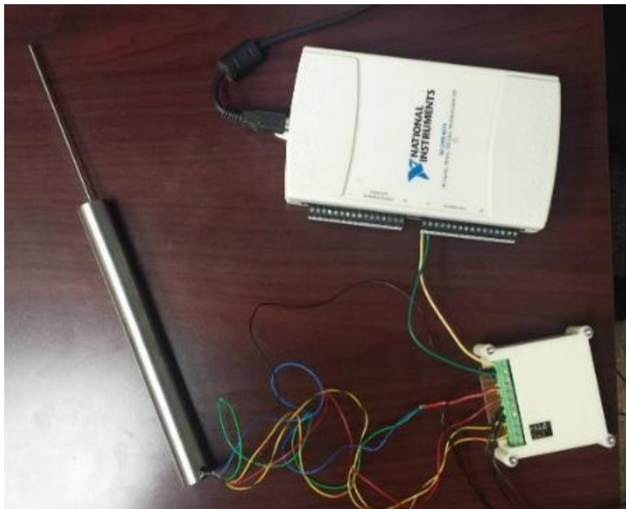
Figure 126: An E-1000 LVDT can detect axial movement with a total span of \pm 1 inch.
