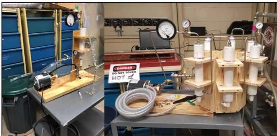
Figure 6: Single and Multiple NF Membrane Bench Scale
