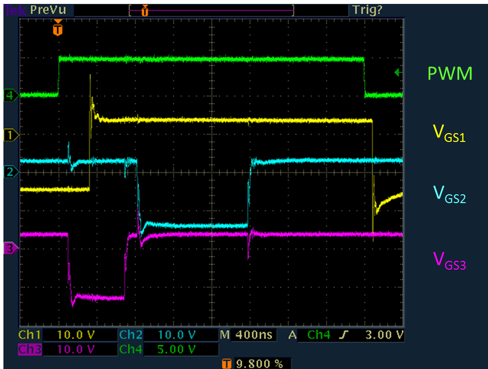
Figure 5.5: Switch cell gate driver waveforms.
