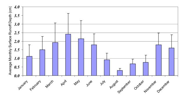
**Fig. 1.** Average monthly surface-runoff depth (cm) and standard error as calculated using daily streamflow data and hydrograph separation using the Base Flow Index software program for nine sub-basins within the Illinois River Basin, Arkansas and Oklahoma.
