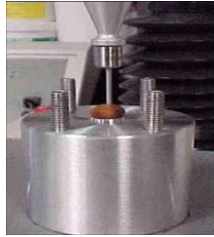
2-mm probe puncture
