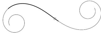
Fig. 1. An Euler spiral, its inflection point (circle) and a Euler spiral segment (black).
