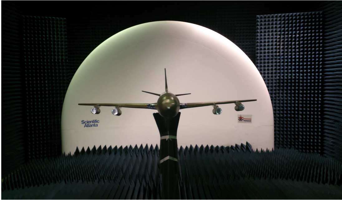
Figure 10.7: Front view of 1:25 scale Boeing 707 model in the University of Pretoria's compact range.
