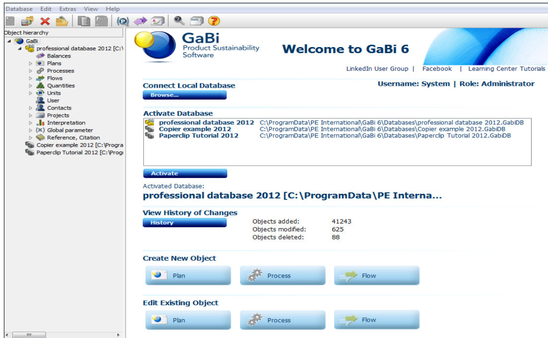
Figure A7 Display page of the GaBi 6.0 software where the database is activated to initiate an analysis.
