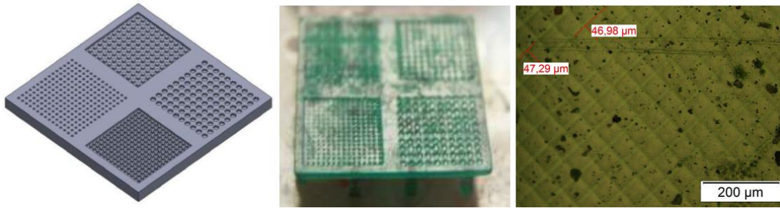
Figure 1. Micro features by DLP part (total part size 7x7x0.5 mm). Pixelation structure due to resolution of DLP. Courtesy University of Las Palmas de Gran Canaria.
