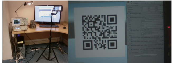
Figure 9: A function generator drives a PPS to a GPIO card where it is used to synchronise the phase of the system clock and an LED visible to the high speed camera. The QR code is undergoing a transition.
