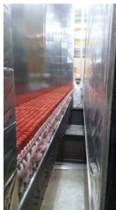
Figure 10. A photograph of the coupling between the first tracker module and the first calorimeter main wall, which took place in October 2016 at the LSM. This completes the installation of half of the instrumented SuperNEMO Demonstrator Module detector.
