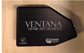
Figure 5.59: Ocean Optics Ventana miniature Spectrometer with enhanced Throughput (F/2)
