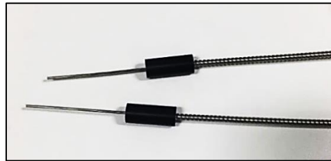
Figure 8.117: Broadband-NIRS source and detector optical fibres designed for reflectance measurement of the retina with small numerical aperture (0.37) and small core diameter (600 \mu\text{m} ).
