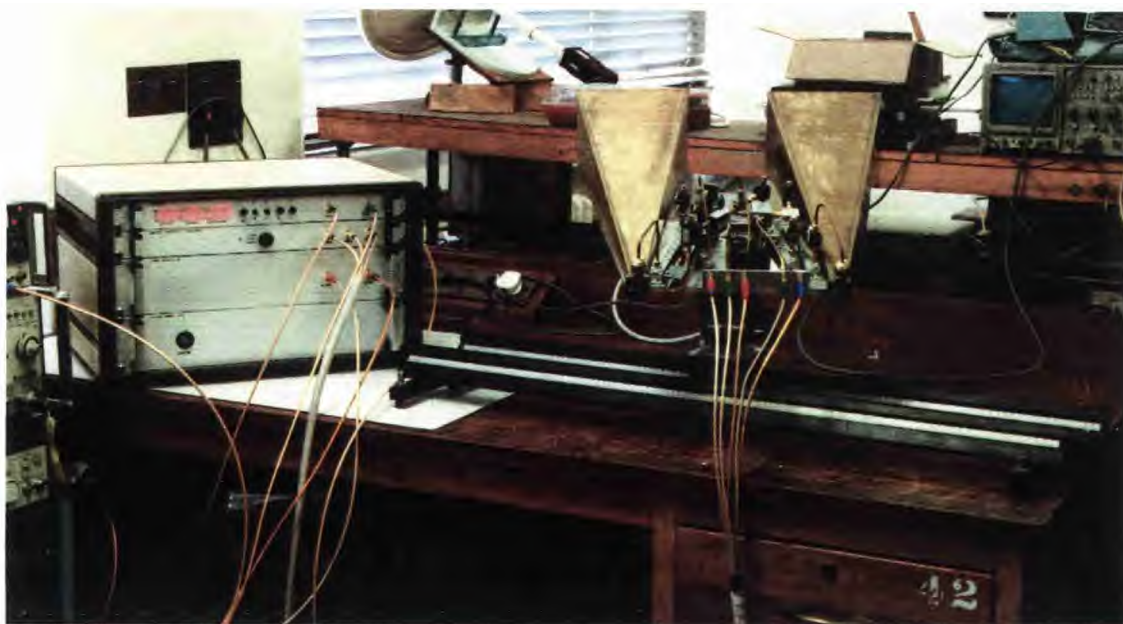
Figure 5.6- Radar rack and microwave head with their cablings
