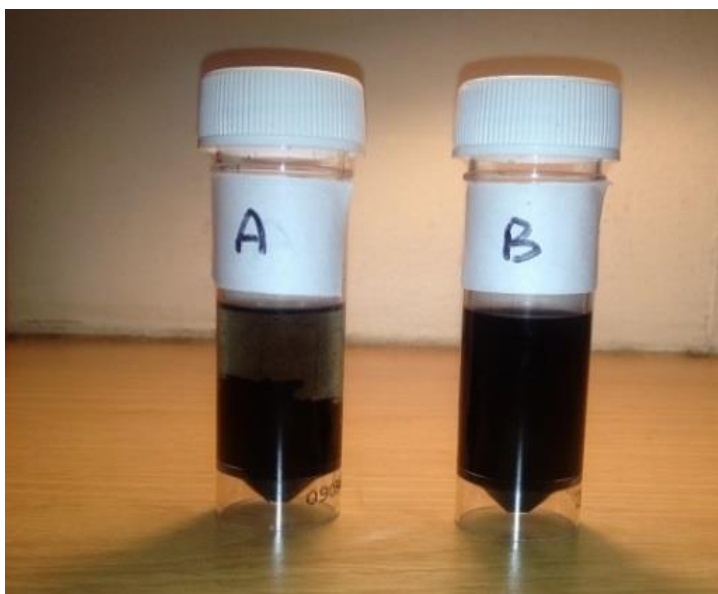
Figure 5-4 Carbon nanotube sedimentation after 2 hours A: unfunctionalised B: functionalised
