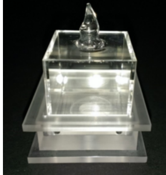
Figure III.5: Cubic Quartz Rubidium Cell. Shape allows for cross-configuration of pump and probe beam.
