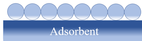
Figure 1-3 Schematic view of monolayer adsorption
