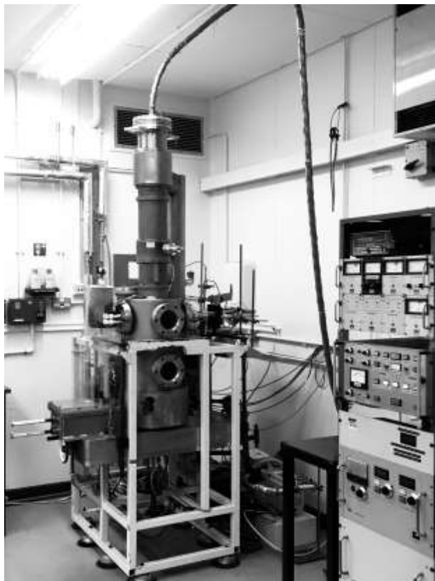
Figure 1. Photograph of the University of York GED instrument described in this article taken during routine operation.
