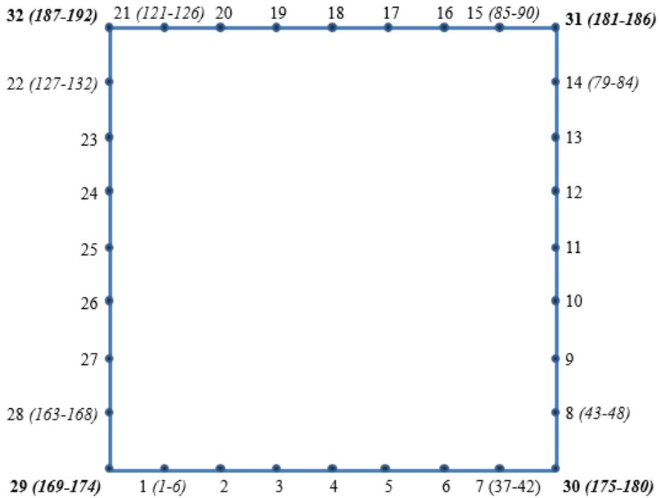
(b) Macro-panel element used by the solver in global analysis. (Numbers in brackets indicate nodal d.o.f.)
