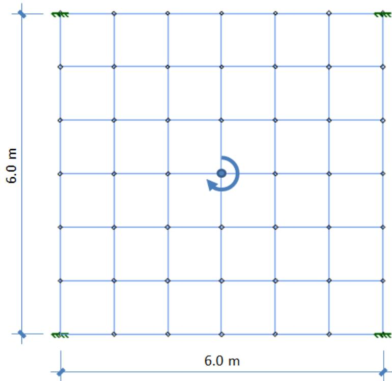
(a) The model (thickness = 0.5 m,  $E = 2.8 \times 10^{10}$  Pa, Moment =  $1 \times 10^6$  N.m)
