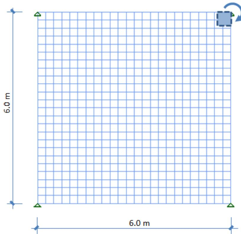
(a) The model (thickness = 0.5 m,  $E = 2.8 \times 10^{10}$  Pa)
