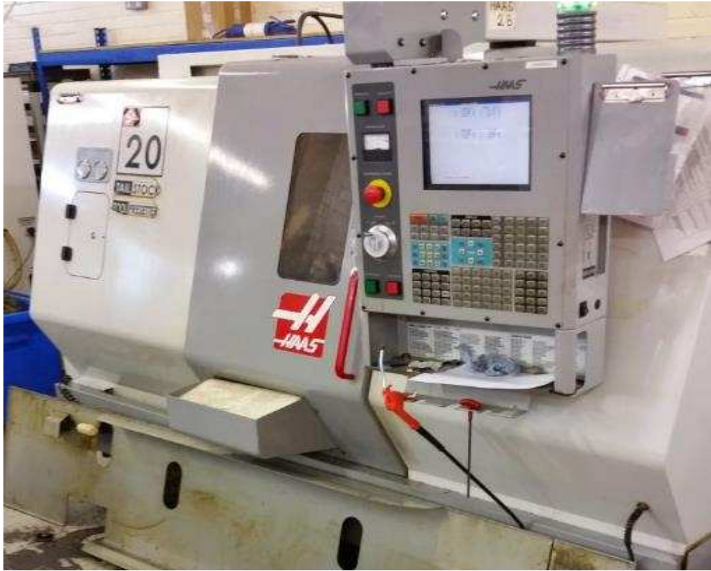
Figure 1.4 - A photograph of an enclosed CNC machine. The machine is operated by external controls, and whilst the machine is in operation, the door remains closed. (The image was supplied by Pennine lubricants Ltd.)
