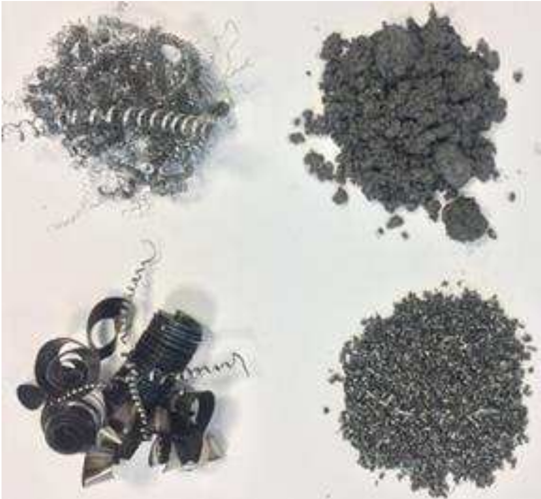
Figure 1.6 – A photograph of the different type of metal particles generated through machining processes. The image shows the different types and sizes of metal fragments and particulates that can be carried away in the MWF during machining processes. The two on the left hand side are defined as swarf. They can vary in size, but can be sharp when handled without protective gloves. These are usually washed away in the MWF. The two on the right are much smaller metal pieces that are formed through grinding processes. They tend to form a thick “sludge” inside the machining tools. Much finer and less visible particles can be generated that circulate in the MWF until filtered out.
