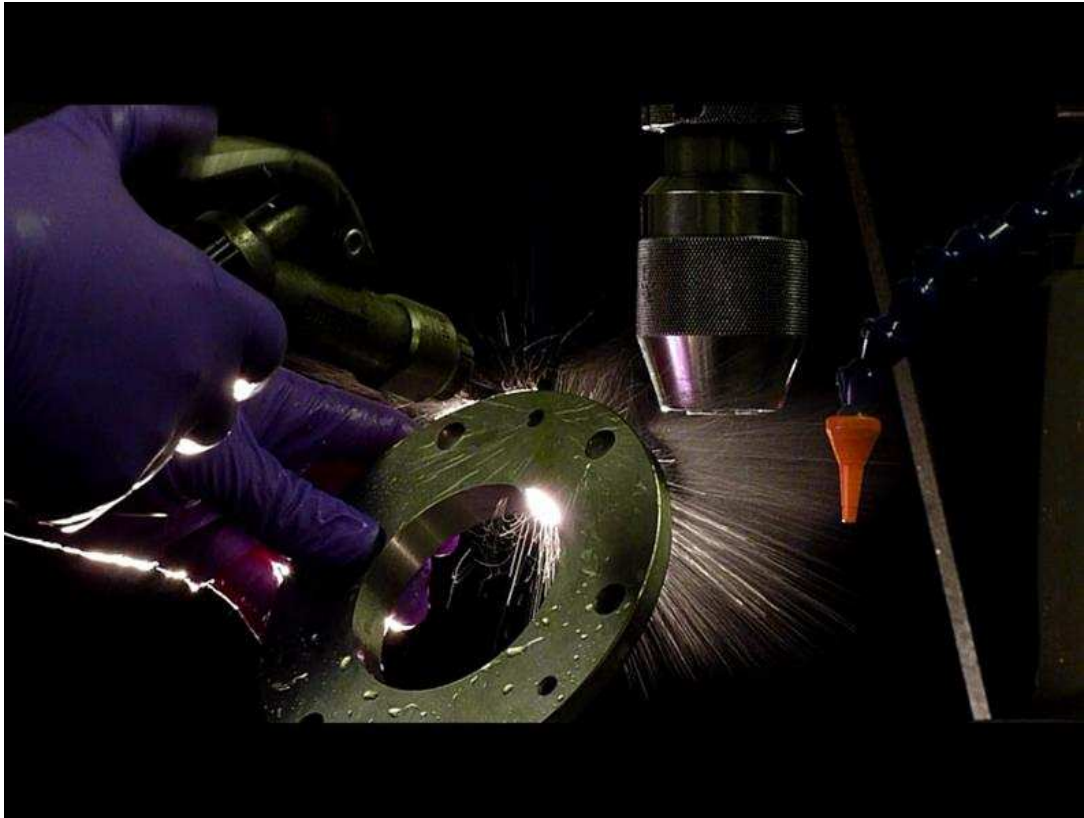
Figure 1.3 – A photograph of a compressed airline being used to blow away the excess MWF on the component. This is the most effective method for cleaning large volumes of components of excess MWF in comparison to a cloth. Therefore, it is common practice in a machining production line. (Image provided by the HSE, UK).
