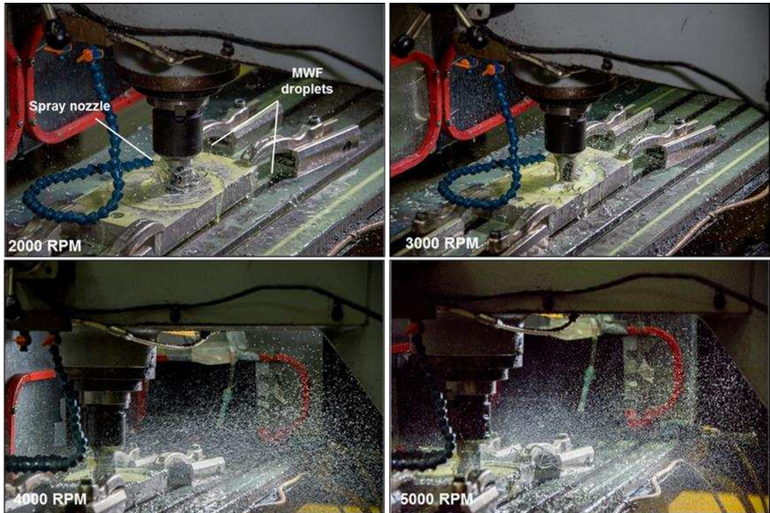
Figure 1.2 – A photograph of a machining tool at rotational speeds increasing from 2000 RPM to 5000 RPM. As demonstrated in the image, the spray nozzle delivery for MWF is directly pointing at the tool. The faster the speed of the tool, the more dispersion of MWF droplets occurs. At higher rotational speeds, the dispersion of the droplets has a further span. Additionally, the droplets are finer. (These images were provided by the Health and Safety Executive)
