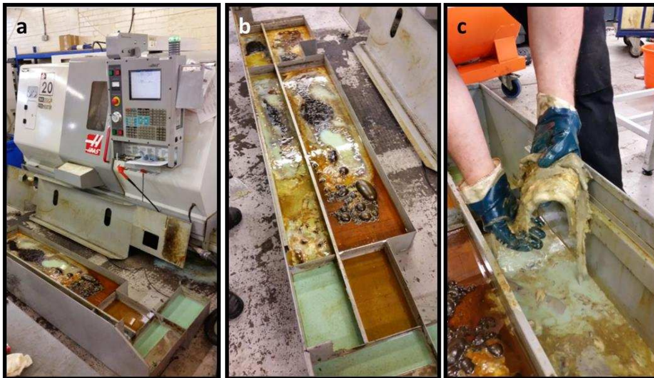
Figure 1.1 – A photograph of a typical well-used and soiled machining tool with sump tank. a.) Is a photograph of a whole machining tool with the MWF sump tank at the front. b.) A close-up image of the machine sump depicting heavy tramp oil contamination floating at the surface. This can be differentiated as the brown substance. The true colour of the MWF is a light blue. c.) Close up image of a solid mass that had formed under the surface of the tramp oil. The individual in the photograph is holding the biofilm that had formed in the sump tank. (The images were supplied by Pennine lubricants Ltd).
