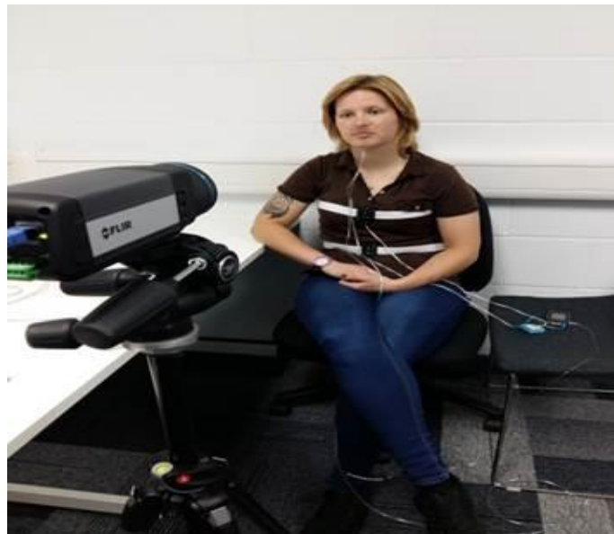
Figure 2 Set-up of the thermal imaging camera during adult testing.
