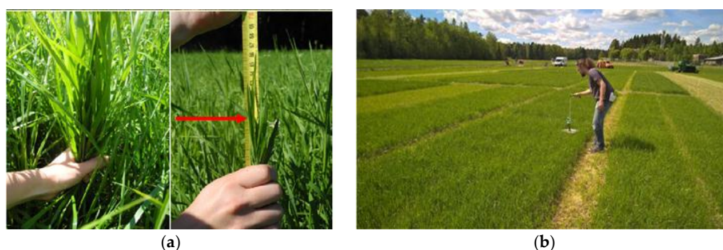
Figure 2. In situ measurements of grass height by: (a) height stick; and (b) plate meter.
