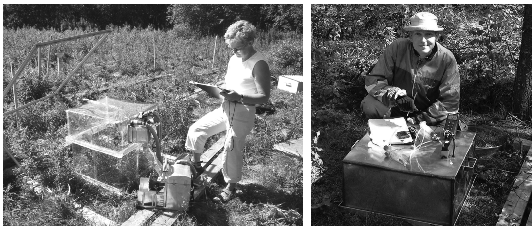
Fig. 1. Closed (vented) chamber systems for measuring \text{CO}_2 exchange NEE between ground vegetation and the atmosphere. Left-hand side panel: the transparent chamber was thermostatically controlled to near ambient air temperature (photo by Miculáš Černota). Right-hand side panel: the opaque chamber was used for total ecosystem respiration R_{\text{TOT}} , and the fluxes of \text{CH}_4 , and \text{N}_2\text{O} . R_{\text{TOT}} was measured with delay after NEE to allow for equilibration of soil \text{CO}_2 conditions (photo by Kees Blom).
