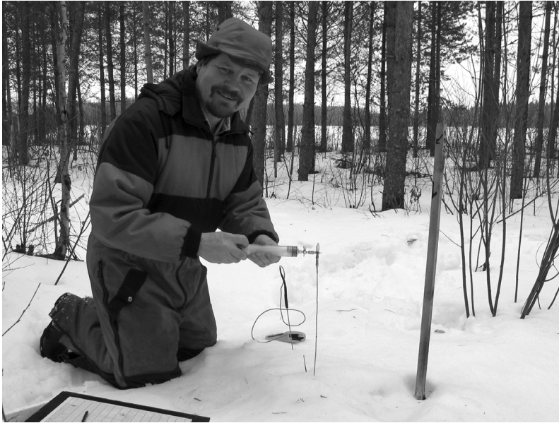
Fig. 4. Gas sampling in snow gradient flux method. A gas sample is taken into a syringe from beneath a known depth in the snow pit, and the gas concentration is compared with that from ambient air above the snow. Snow porosity is measured from a volumetric sample with help of solid ice density. Photo by Markku Parhiala.
