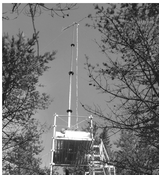
Fig. 2. Eddy covariance tower used to measure gas fluxes at a forested peatland site. Photo by Tuomas Laurila.
