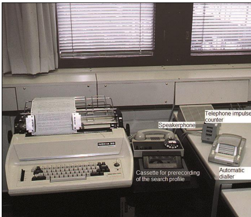
Figure 1.6 A terminal with accessories for accessing online services at VTT Information Service at VTT Technical Research Centre of Finland in the 1970s.
