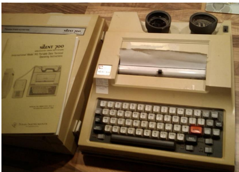
Figure 3.2 Texas Silent 700 printing terminal with acoustic coupler.
