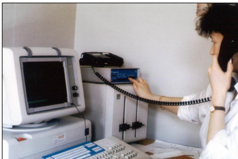
Figure 6.13 IBM word processor IBM Series/80 including a floppy disk drive for two 8 inch floppy disks. On top of the disk drive is a modem capable of communicating at 1,200 bps. Here operated by Ulla Bakker of DAFA, it was mainly used for producing legal texts and uploading these texts to the mainframe computer of DAFA, in order to update the databases of the online legal service Rättsbanken. It could also be used for accessing online services, including searching as well as downloading and storing of search results (which were very advanced options for that time). Photo: Lars Klasén, 1986.
